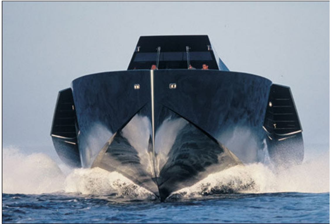
The hull form is a deep V of 22 degrees at the stern, with a straight stem bow designed to perform a wave piercing.
